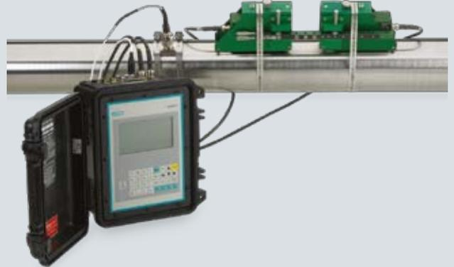
The energy meter family with its rugged and high precision characteristics is ideally suited for thermal energy and power applications, and is particularly suitable for large pipe sizes.
